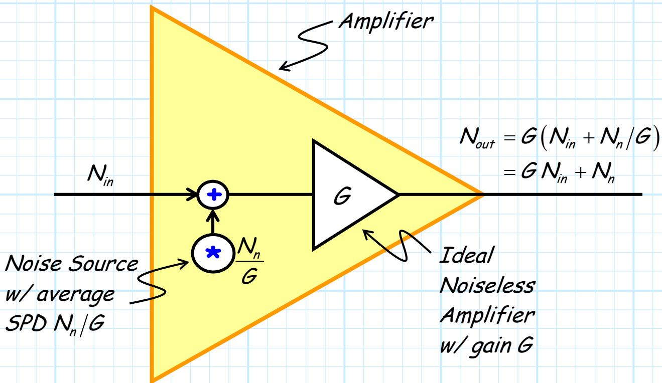
Note here that the noise source near the **input** of the amplifier has an average spectral power density of  $N_n/G$ .
