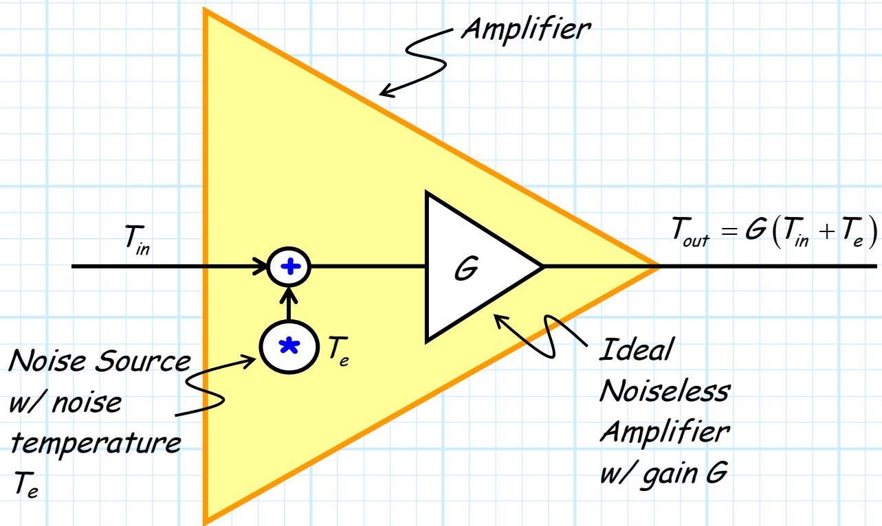
$$T_{out} = G(T_{in} + T_e)$$
