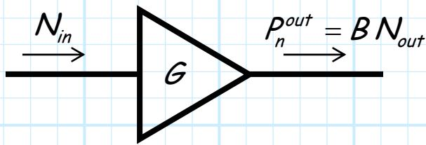
Here there is no input signal at the amplifier input, other than some **white** (i.e., uniform across the RF and microwave spectrum) **noise** with average spectral power density  $N_{in}$ . At the **output** of the amplifier is likewise noise, with an average spectral power density of  $N_{out}$ .
