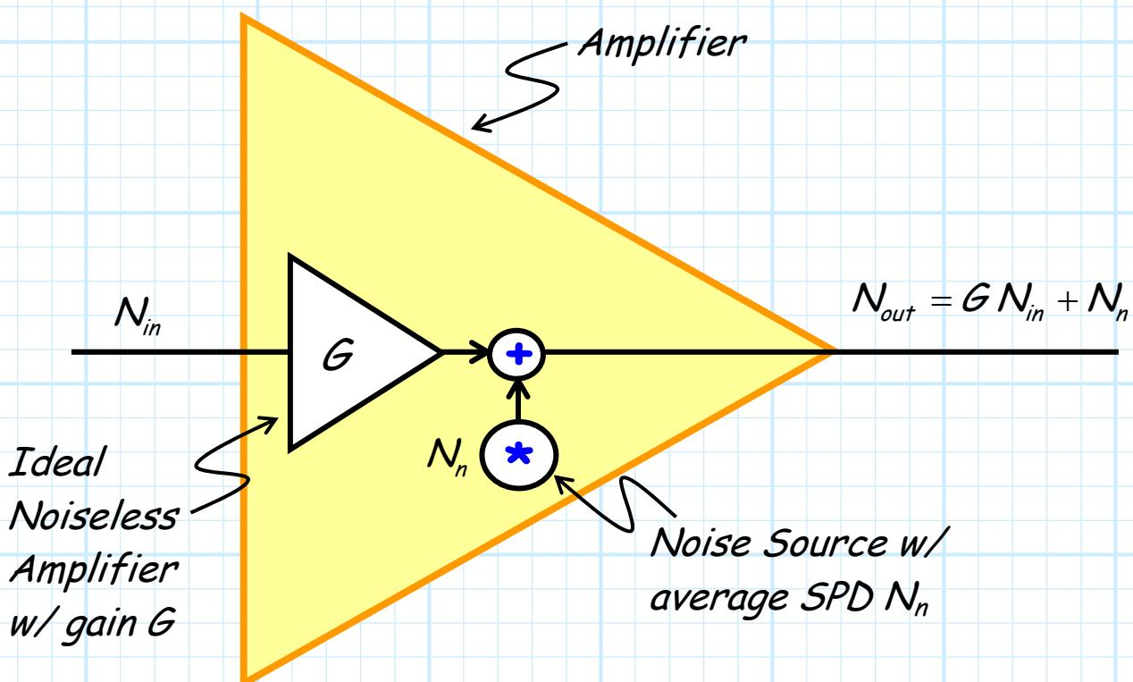
Note however that this is **not the only** way we can model internally generated noise. We could **alternatively** assume that **all** the internally generated noise occurs near the amplifier **input**—and thus **all** this noise is amplified with gain  $G$ !
